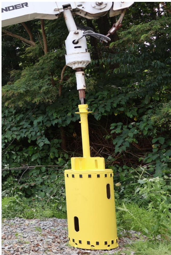
Our 26" stowable stand-alone core barrel.
